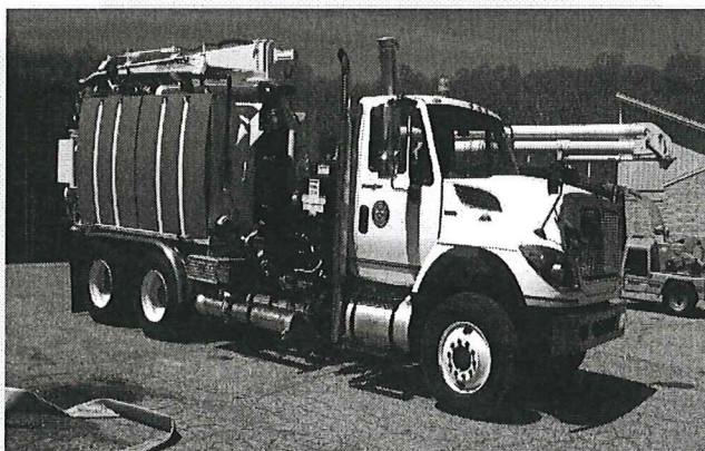
Pipeline Vacuum and Jetting Truck
