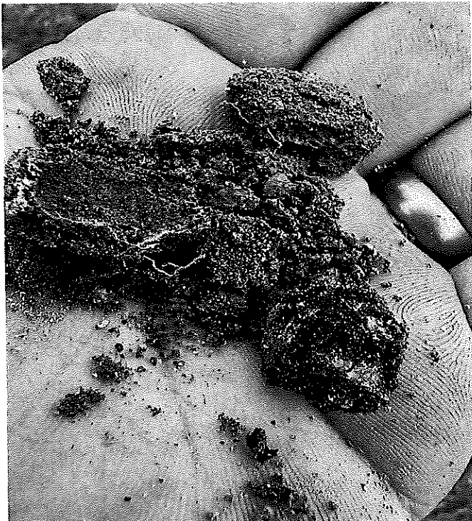
Photo 3: A small asphalt chunk within the top 5".
