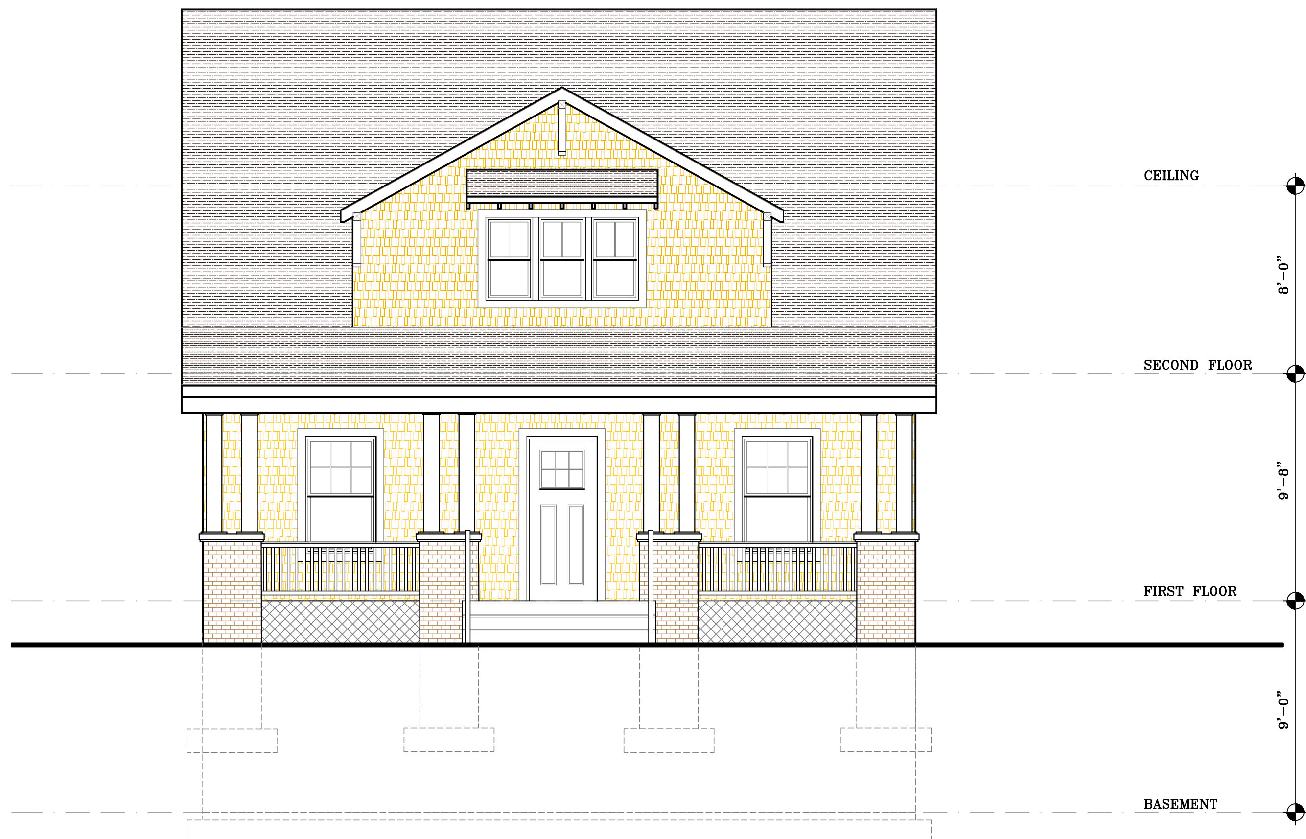
1 WEST ELEVATION SCALE: 1/4" = 1'-0"
