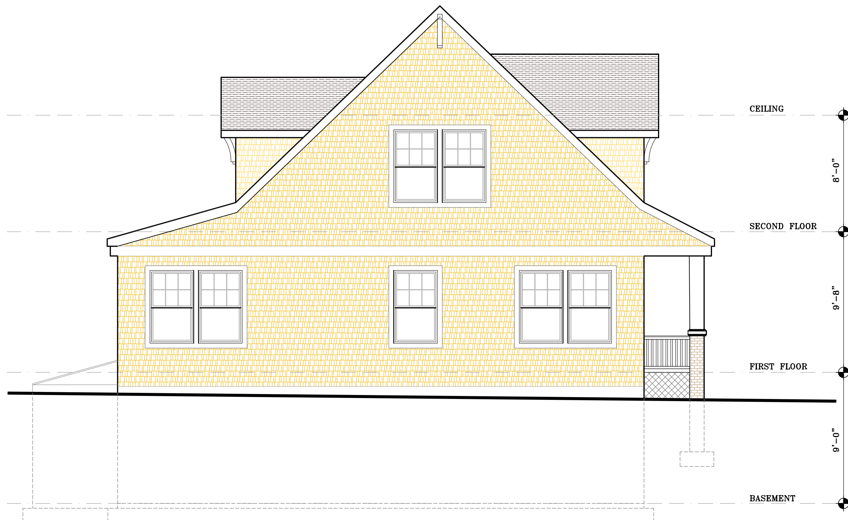
3 NORTH ELEVATION SCALE: 1/4" = 1'-0"
